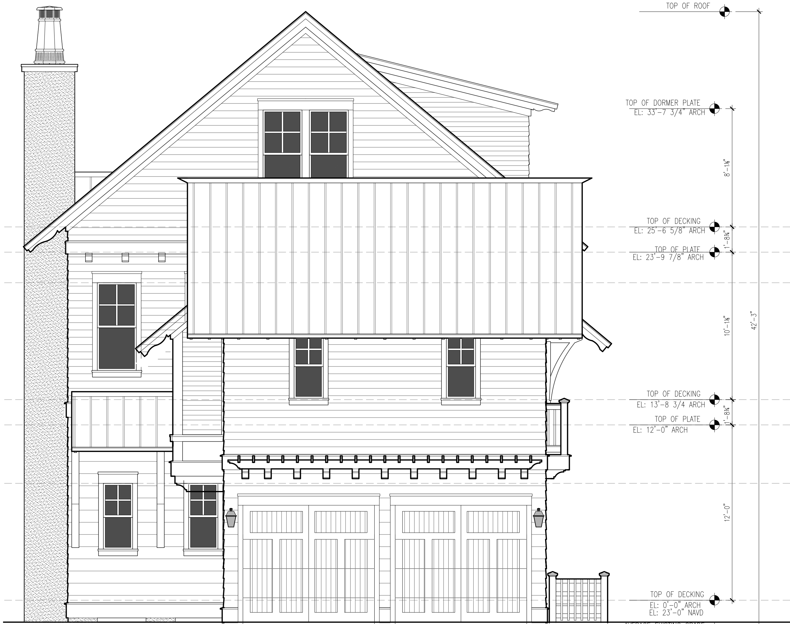
2 REAR ELEVATION SCALE: 1/4" = 1' WHEN PLOTTED AT 24 X 36
