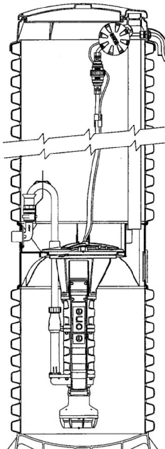
The DH071 is the "hardwired," or "wired," model where a cable connects the motor controls to the level controls through watertight penetrations.
