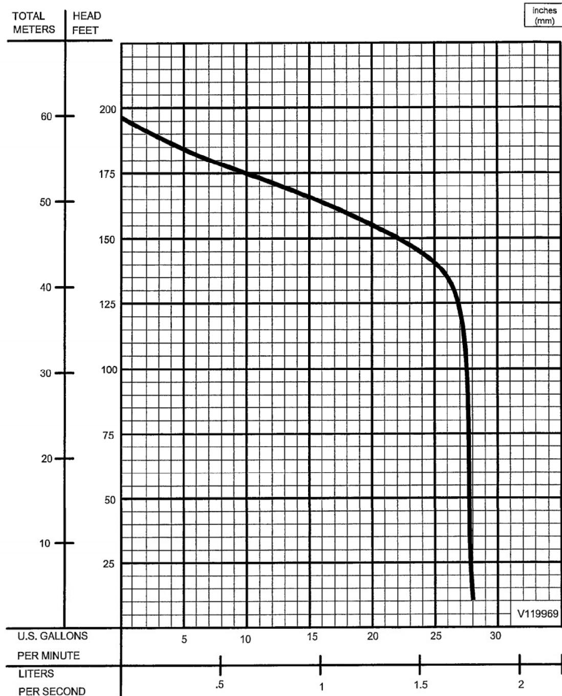
Performance curve includes impact of integral anti-siphon and check valve.
