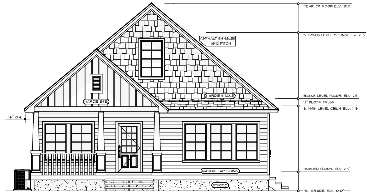
FRONT ELEVATION SCALE: 1/4" = 1'-0"
