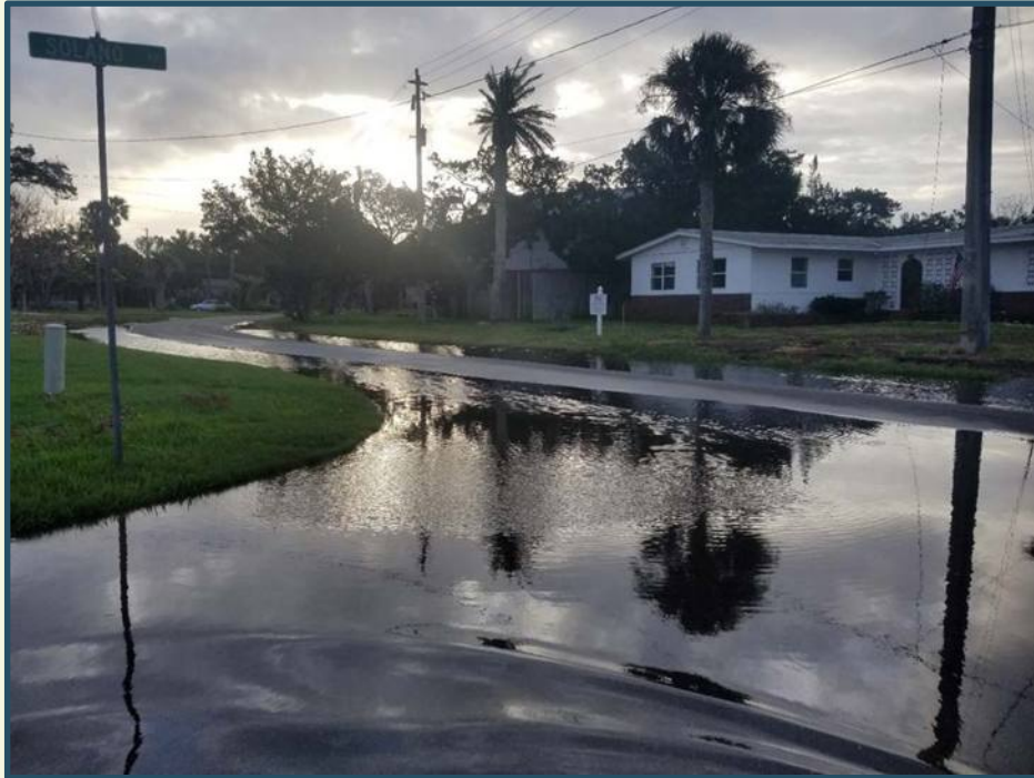
OF-0117 (Before): street flooding during King Tide event (October 2017) due to non-functioning valve
